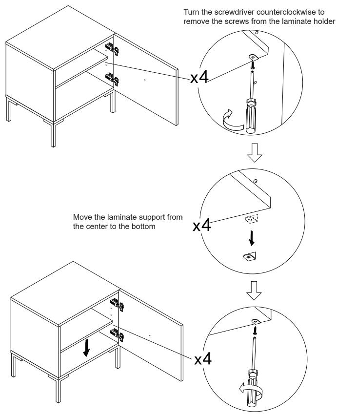
Turn the screwdriver clockwise to screw in the laminate holder
