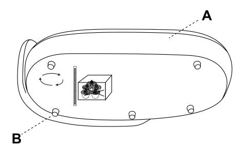
> Position the product bottom-side up and simply screw the legs into the pre-drilled holes as illustrated.
