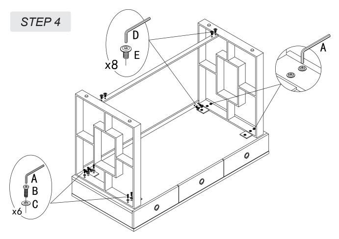
Once the legs have been installed to the body , all screws should be fully tightened
