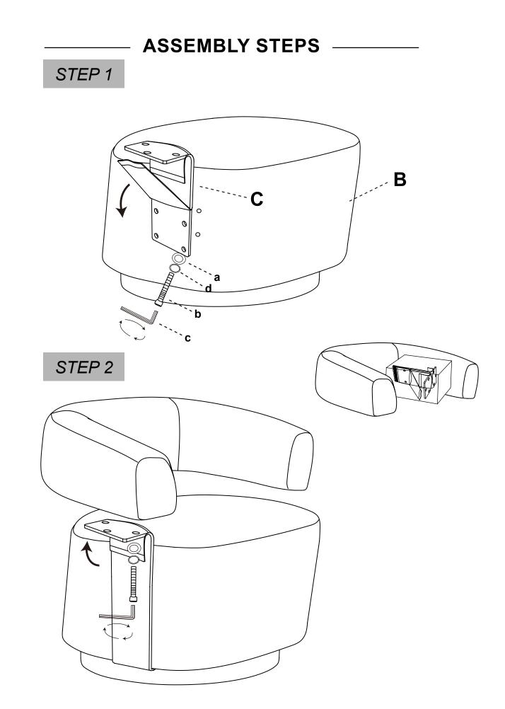
> Use the included hardware to assemble the backseat.
