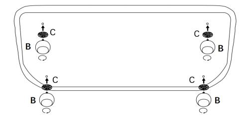
Install the legs by threading them into the pre-drilled holes as illustrated.
