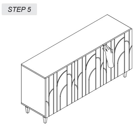
The door can be opened by pressing the corner of the panel
