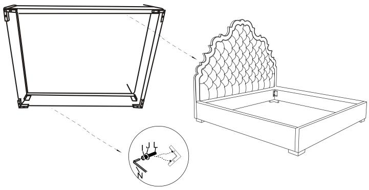
STEP 3 Attach the 3 support legs to the support bar and ensure all legs are securely attached.
