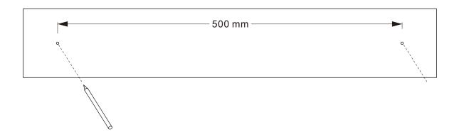
STEP 2: Drill the holes into the wall .
