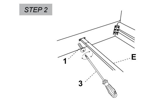
>Attach the center support bar as shown.
