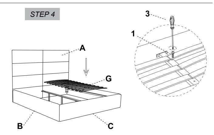
> Screw the bolts (1) into the pre-drilled holes on the support bar to secure the slats in place.
