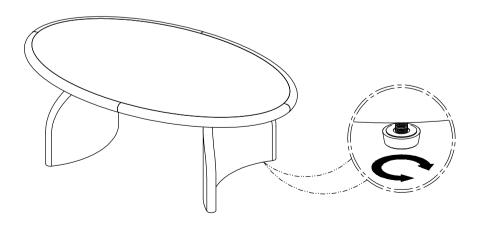
The floor glides can be adjusted to ensure the table's stability
