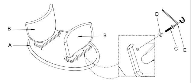
Using the included hardware, attach the tabletop to the pedestal base as illustrated
