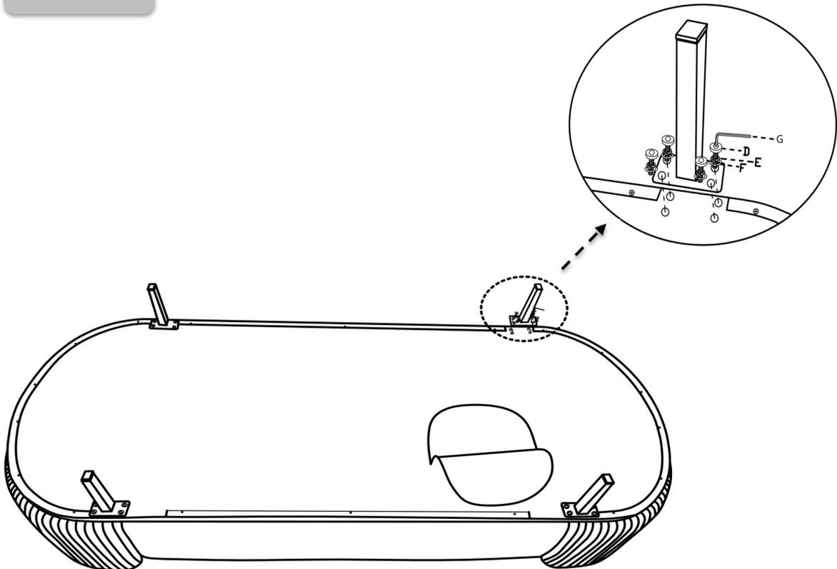
> Position the legs as shown and use wrench to tighten screws clockwise into the pre-drilled holes to attach the leg.
