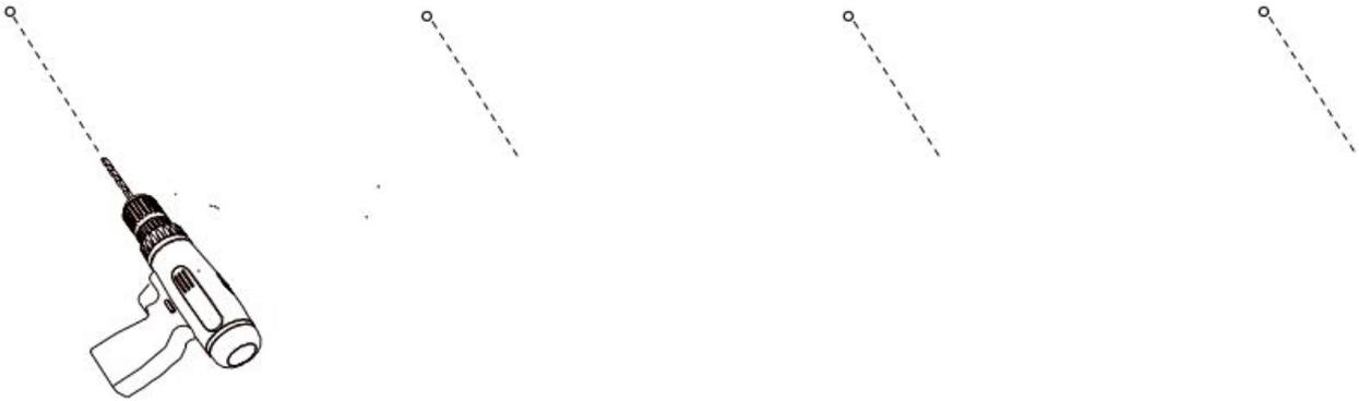
STEP 3: Install the included anchor (B), cleat (D) and screw (C) to the wall. The mirror can now be hung as illustrated.
