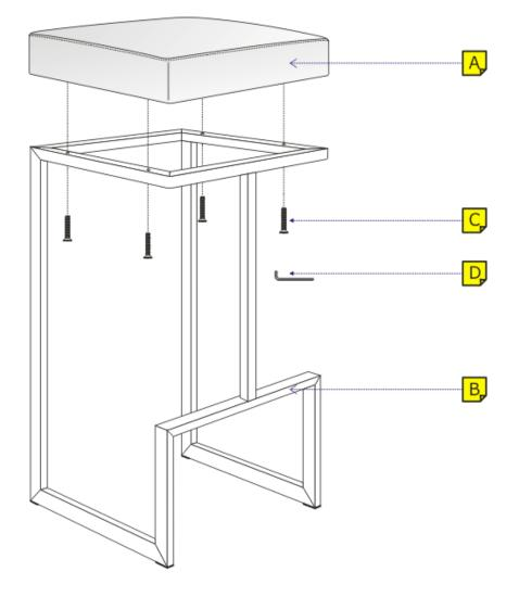
As the picture shows. Tighten the screws.
