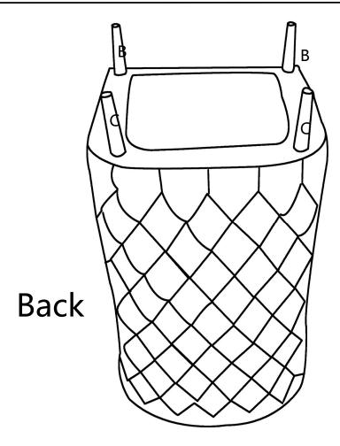
Install leg into the chair by insert the threaded stem into the threaded Hole at each Corner of the bottom of the chair. Tighten by turning leg clockwise. Repeat the same step to install the other leg
