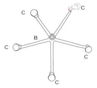
Attach the five Casters(C) to the Chassis as shown.
