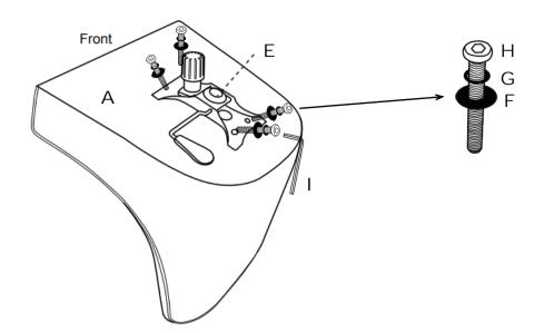
Connect the Lever Mechanism(E) to the Chair body (A) as shown.
