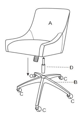
Connect the Chair body (A) and the assembled base with the Gas lift (D) as shown. Assembly is complete.
