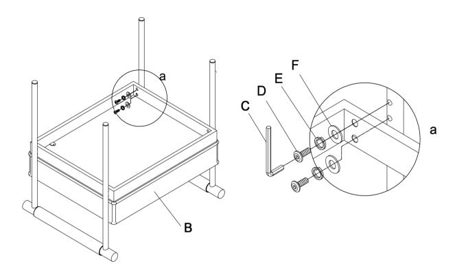
>Attach the Seat to Armrests using the included hardware as shown.
