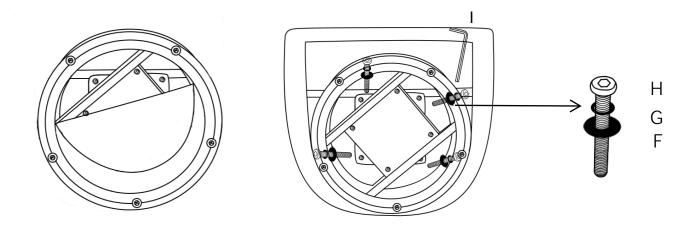
) use provided hardware to attach to the pre-drilled holes on the chair frame.
